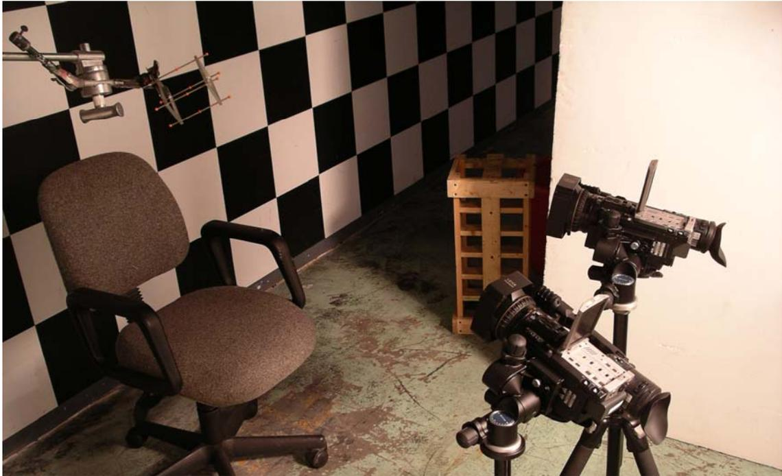
*Figure 7.7 Physical setup for the Regina data set. Notice the tracking cubed placed where the head of the actress will be located. The tracking cube was used to track the cameras with respect to each other and the scene.*
