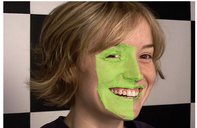
Figure 1: Deforming polygonal mask accurately tracking the subject's face using Model Flowing from 3 camera views.
