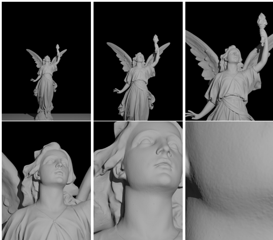
Figure 14.1: Zooming in on The Lucy model ( 3000 \times 1726 \times 5144 ) using the DT-Grid as the underlying level set representation. The pictures demonstrate the high detail present in the model. Note that the bumps on the surface as seen from the closest viewpoint are not artifacts from the scan conversion process, but rather very fine scale detail also present in the corresponding mesh representation generated from scanned real world geometry. Renderings by Ola Nilsson based on my scan conversion.
