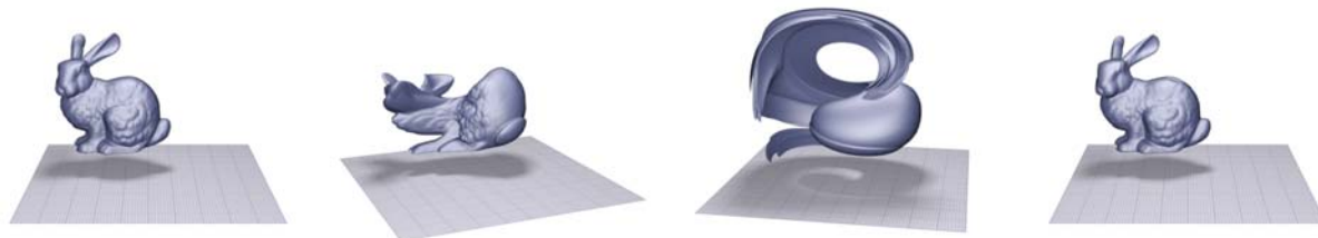
Figure 15.1: Extreme level set deformation of a high resolution model resulting in very thin walls during the course of the simulation. The Stanford bunny is advected by a divergence free and periodic vector field [35, 75] and returns to its original shape after one period, provided the simulation is run at sufficient resolution. The maximum bounding grid is 1024^3 , but memory requirements of the H-RLE grid never exceed 97MB. From left to right the simulation times are (in units of the period) 0, 1/15, 1/2, 1. Rendering by Ola Nilsson based on my simulation data. Stanford Bunny courtesy of the Stanford Scanning Repository.
