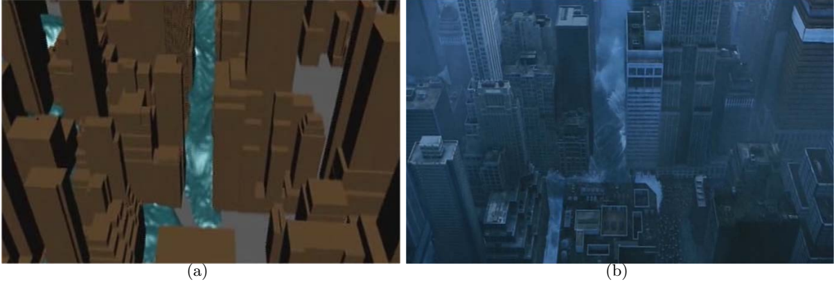
Figure 1.2: This figure shows two stages in the creation of a shot from “The Day after Tomorrow”. ©Twentieth Century Fox. (a) The raw low resolution output from the level set based fluid simulation. (b) The final composite with particle and texturing effects applied.
