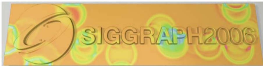
Figure 15.7: The wave equation on a Siggraph plaque. Resolution of model 1024 \times 250 \times 50 . The wave is visualized by color coded surface properties. Rendering and simulation by Ola Nilsson.
