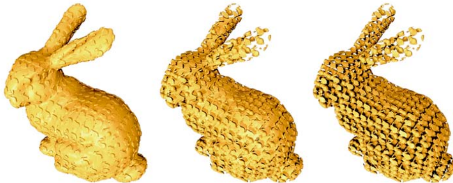
Figure 10.9: Level set morph between a 2048^3 bunny (304MB) and a highly detailed level set CSG bunny (1.62GB) modeled as an out-of-core CSG intersection of the 2048^3 bunny (304MB) with a tiling of 20^3 smaller bunnies each at resolution 128^3 (7.47GB). Reported sizes are in uncompressed DT-Grid format. Peak storage requirements for the morph are close to 5GB.
