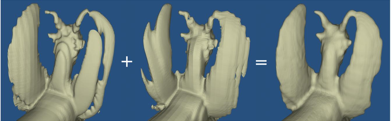
Figure 1: 3D level set model of a griffin derived from two non-uniform laser scan reconstruction volume datasets. The two input models with resolution  $294 \times 312 \times 24$  and  $294 \times 52 \times 144$  show severe aliasing effects from insufficient sampling, especially in the wings. Our method merges information from both of the datasets to produce a high resolution  $294 \times 312 \times 144$  level set model. All models throughout this paper are flat-shaded to highlight details.
