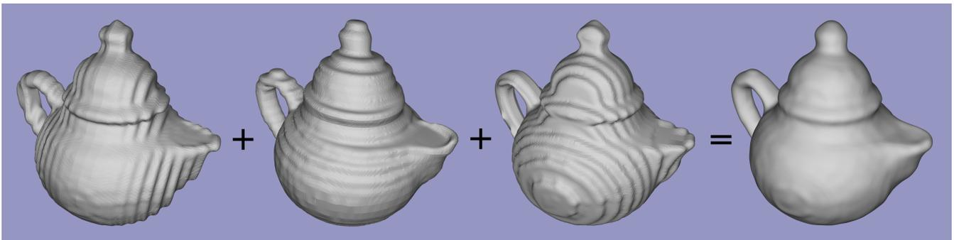
Figure 6: Three non-uniform samplings of a high resolution CT scan of a teapot, followed by a level set model derived from the first three scans.
