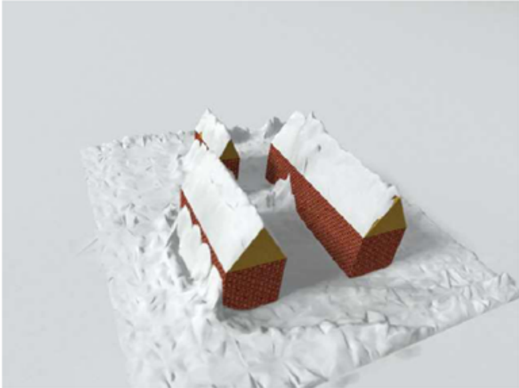
Figure 4.6: Feldman scene as presented in [MMA+05]. Snow-cover is not very smooth. Sharp edges, uncharacteristic of snow, reveal the underlying triangulation.
